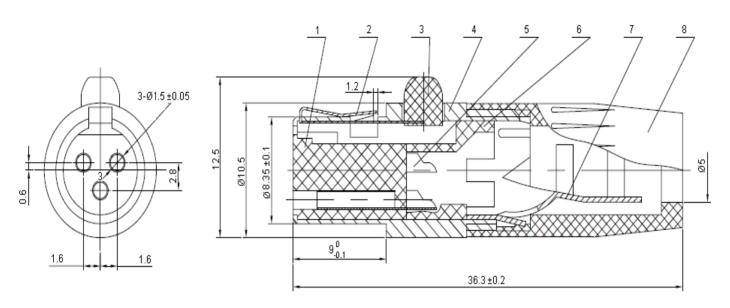
The female pin plating gold, Thickness 0.05 μm (Solder)
