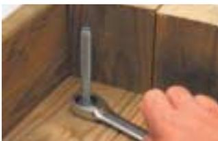
Works in places even deep sockets won't reach. It's the perfect tool for positioning and tightening bolts on threaded rod adjusters like those found on most electric garage door openers.
