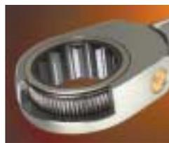
The box end ring gear has 72 extra-fine teeth, allowing the ratchet mechanism to engage with just a 5° movement of the wrench. This important component is precision machined and specially heat-treated for exceptional strength.
