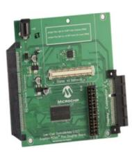
The Low-Cost Controllerless (LCC) Graphics PICtail Plus Daughter Board enables development of graphics solutions without an external graphics controller, thus reducing system BOM cost for many applications. The board is designed to attach to a PIC32 starter kit (DM320001, DM320003-2, DM320004) or an Explorer16 development board (DM240001) and one of Microchip LCD Modules including the Truly 3.2" QVGA board and the 4.3" WQVGA Powertip display panel
