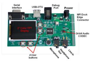
The audio board can be easily connected through the MFi dock edge connector to the <u>accessory development platform for</u> <u>iPod and iPhone</u> enabling users to develop applications for iPod and iPhone.
