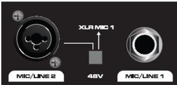
Connect microphones, DI boxes and other balanced low impedance audio inputs to the MIC/LINE combo inputs using good quality XLR leads. Alternatively, connect high impedance and line level signals to the combo inputs using 6.3mm jack leads. (+ additional rear jack input for MIC/LINE 1). If phantom power is to be used for condenser mics, press “+48V” switch and connect using balanced XLR cables.
