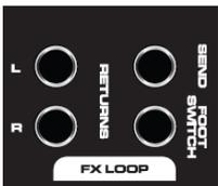
If the internal DSP reverb effect is to be operated remotely, connect a latching foot switch to the rear panel F/S jack. Alternatively, this can switch the feed from an external unit, which should be connected via the FX LOOP. To do this, connect a jack lead from the SEND to the external effect unit and its left & right outputs to RETURN L+R.
