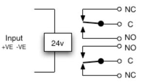
This relay is polarised and is therefore suitable for alarm bell circuits. It must be wired the correct way round for it to operate. There is also a back EMF suppressing diode.
