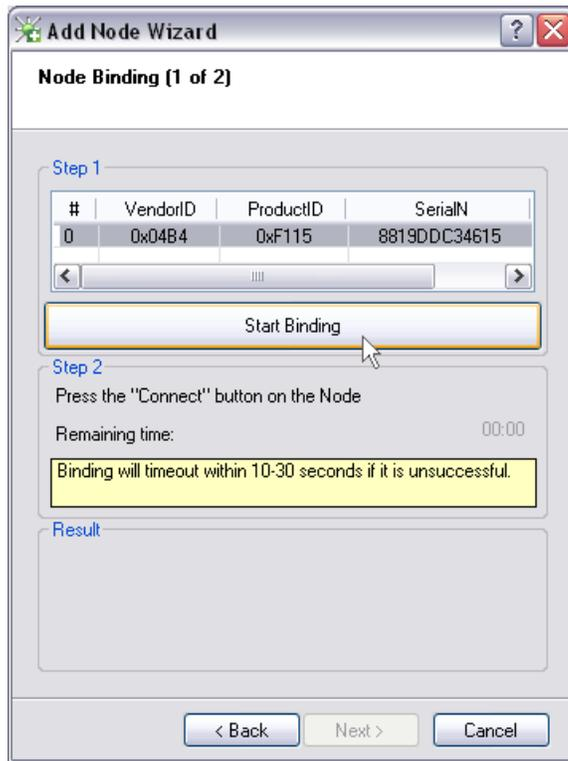
13. After activating this function, you have approximately 10 to 30 seconds to press the bind button on the RF expansion card.
