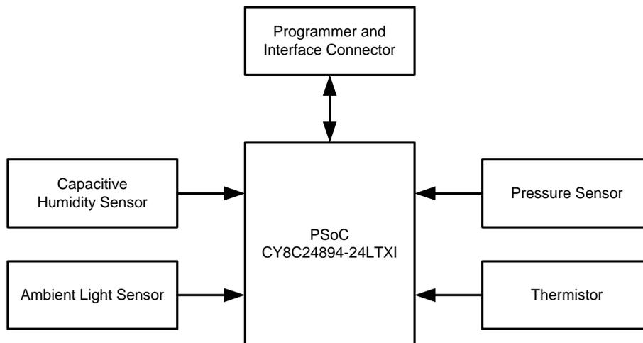
Figure 3-2. Weather Station Expansion Board
