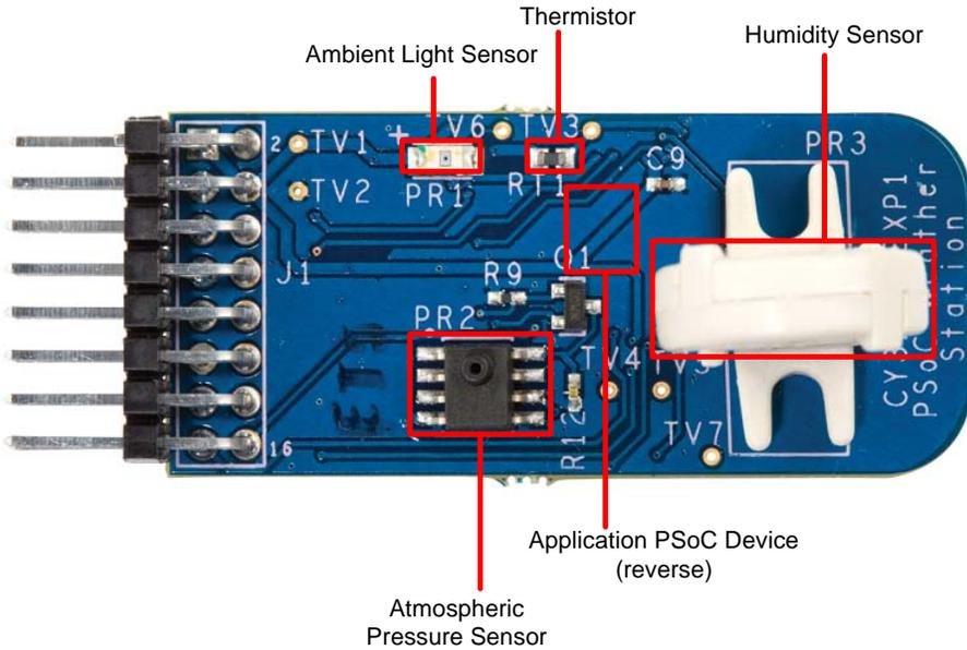
The weather station expansion board sends sensor data over I2C to the RF expansion card, which is included in the CY3271-FTRF kit.
