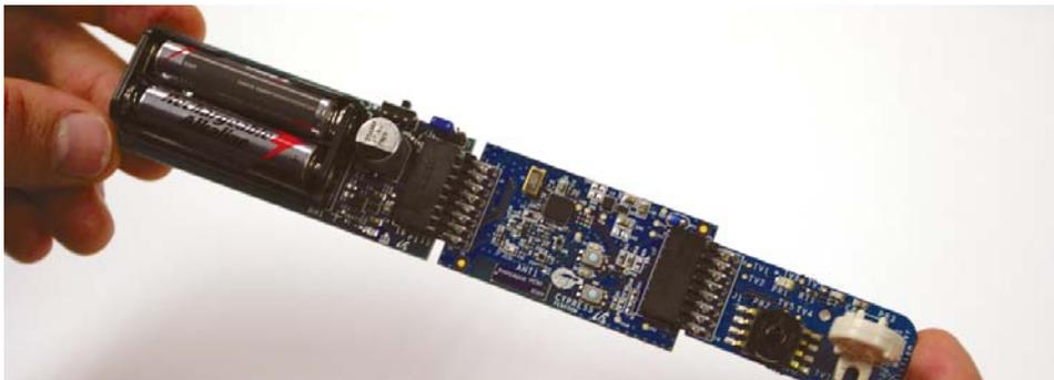
7. Power the RF expansion card by sliding the ON/OFF switch on the battery pack towards the card.
