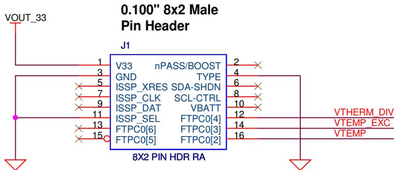
**NOTE: This Expansion Board Does Not Have An Onboard Voltage Regulator - DO NOT Power With > 5Vdc**
