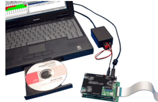
Compact emulator for the H8/300H Tiny series
