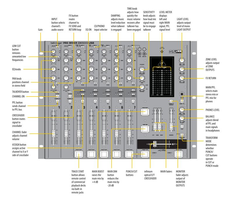
CUT mode enables the big buttons to be used as mutes for interesting gating effects, temporarily silencing the X or Y output. In PUNCH mode the X button introduces the X signal to the mix, while the Y button brings in the Y signal. This means you can add in bits and beats from X on top of Y and vice versa, opening up your scope to extremely creative mixing.
