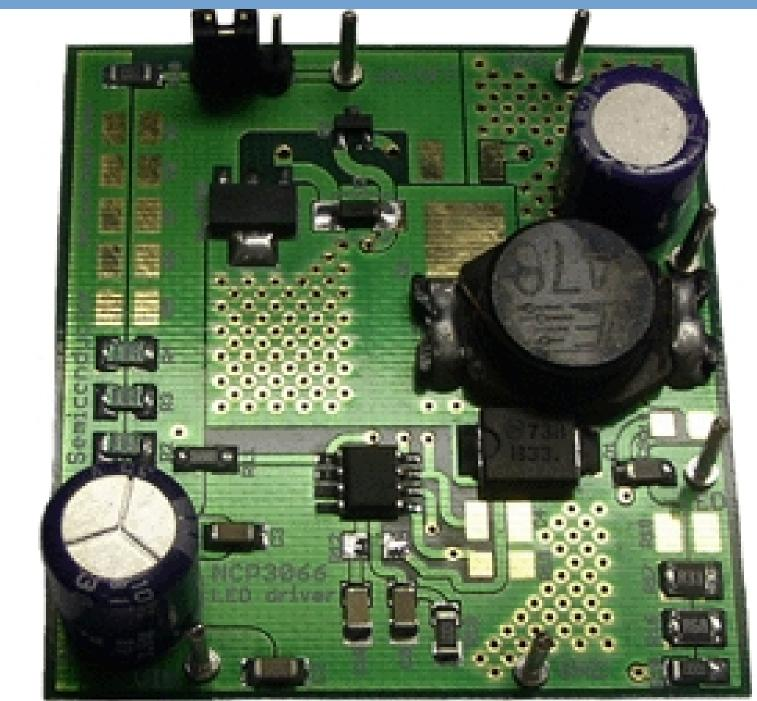
1.5Å with a maximum duty cycle of 85.7%. The ON/OFF function allows turning of the device to low consumption mode, or driving the LED brightnes using PWM signal. The NCP3066can also be used as a controller for peak currents greater than 1.5Å when an external device is used. Size: 53mm x 50mm x 14mm
