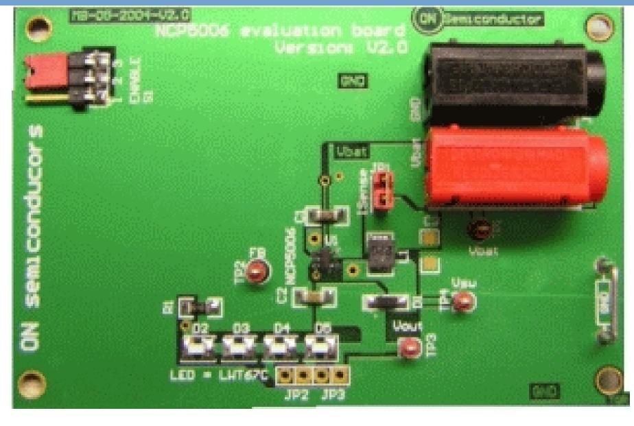
optimized for small ceramic capacitors, capable of supplying 1.0 W output power.
