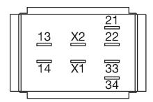
Series > 01 > Accessories > Front > Lens plastic > 61-8490.12 - Switching element for pushbutton and keylock- and selector switch 2 pose a O Stand: 13.02.2012
