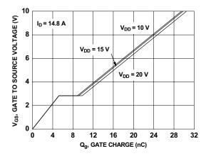
Figure 7. Gate Charge Characteristics
