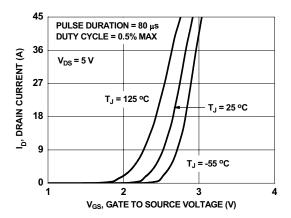
Figure 5. Transfer Characteristics
