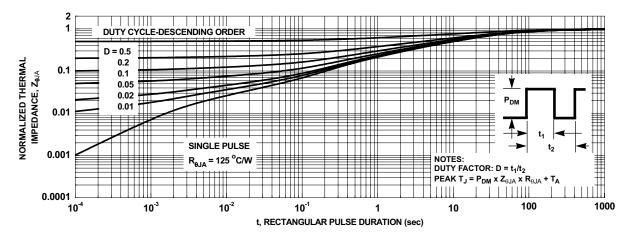
Figure 12. Junction-to-Ambient Transient Thermal Response Curve
