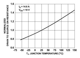
Figure 3. Normalized On-Resistance vs Junction Temperature
