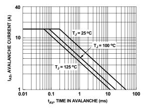
Figure 9. Unclamped Inductive Switching Capability
