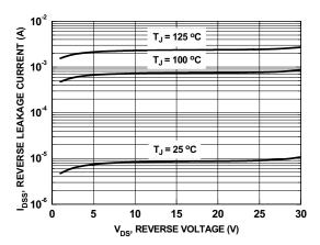
Figure 14. SyncFET body diode reverses leakage versus drain-source voltage
