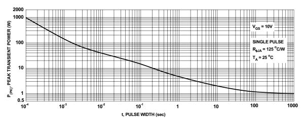
Figure 11. Single Pulse Maximum Power Dissipation
