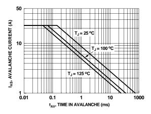
Figure 9. Unclamped Inductive Switching Capability
