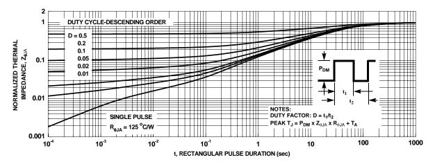
Figure 13. Junction-to-Ambient Transient Thermal Response Curve
