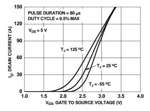
Figure 5. Transfer Characteristics
