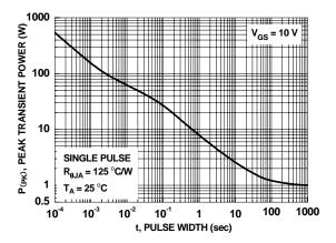
Figure 12. Single Pulse Maximum Power Dissipation
