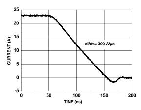
Figure 14. FDMS7572S SyncFET body diode reverse recovery characteristic
