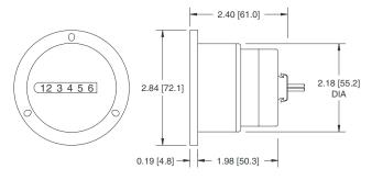
Mounting holes: For #4 screws on 2.44" [62.0] B.C. and #6 screws on 2.53" [64.3] B.C. Panel cutout: 2.21" [56.1] Dia.
