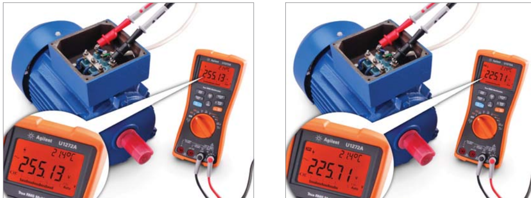
Figure 2: Comparison of voltage output from industrial motor VFD without and with Low Pass Filter functionality.
