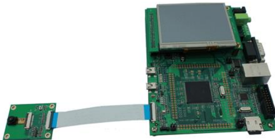
CAM1207 connects to DevKit1207 board
