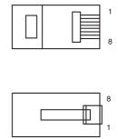
The connection at the DCM-I end is identical. Note that the CAT-5 interconnection provides DC power as well as data, but also see the following chapters concerning connecting and mounting the CDR-I and CDRIF.
