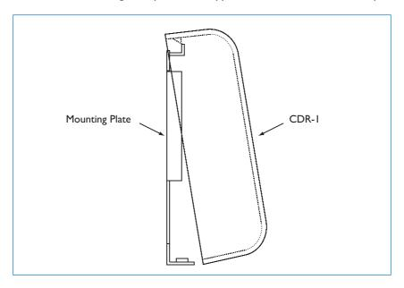
8. Screw the CDR-I to the mounting plate using the two countersunk M3 screws removed in step I.
