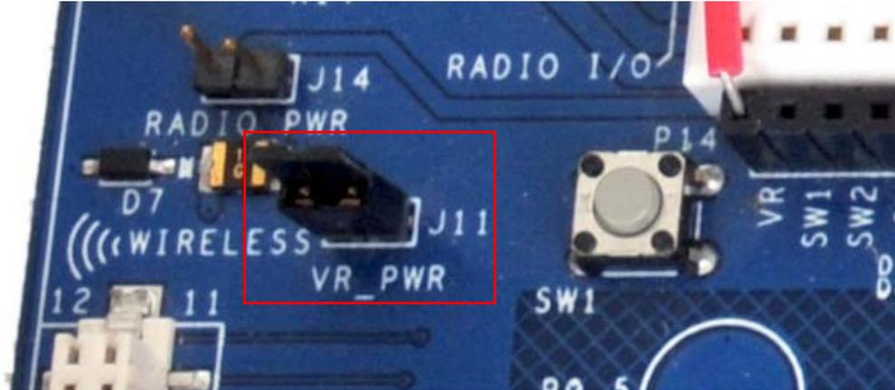
The remaining jumper settings on the DVK are in the default state. See the *PSoC Development Kit Board Guide* for the default setting of jumpers.
