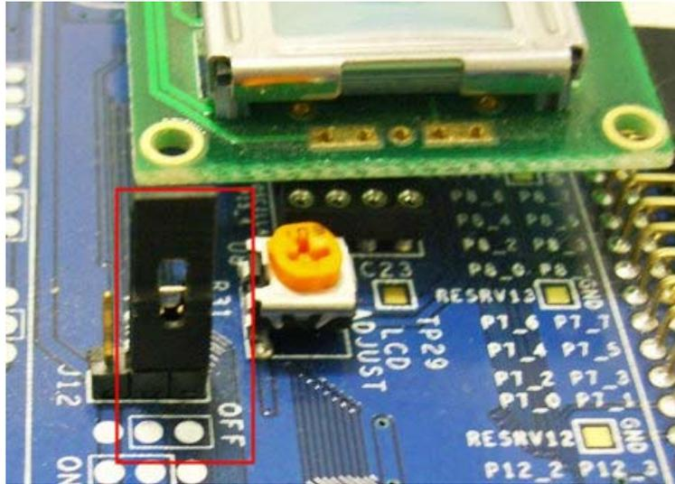
PSoC 3 provides serial wire debugging (SWD) with SWD on GPIO pins option. The port pins used for SWD are P1\_0 (SWDIO) and P1\_1 (SWDCK). Port B uses the P1\_0 and P1\_1 for Seg9 and Seg8 signals, respectively. Therefore, the debugging option is not available when using Port B. PSoC Creator allows routing P1\_1 and P1\_0 to be used as GPIO pins when debugging is disabled. To disable debugging, follow these steps:
