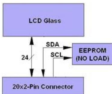
This board includes a custom LCD glass with maximum 128 segments. The glass has 24 pins (8 common and 16 segments lines) that are routed to the 20x2 pin connector and connected to the configured I/O pins of PSoC 3.
