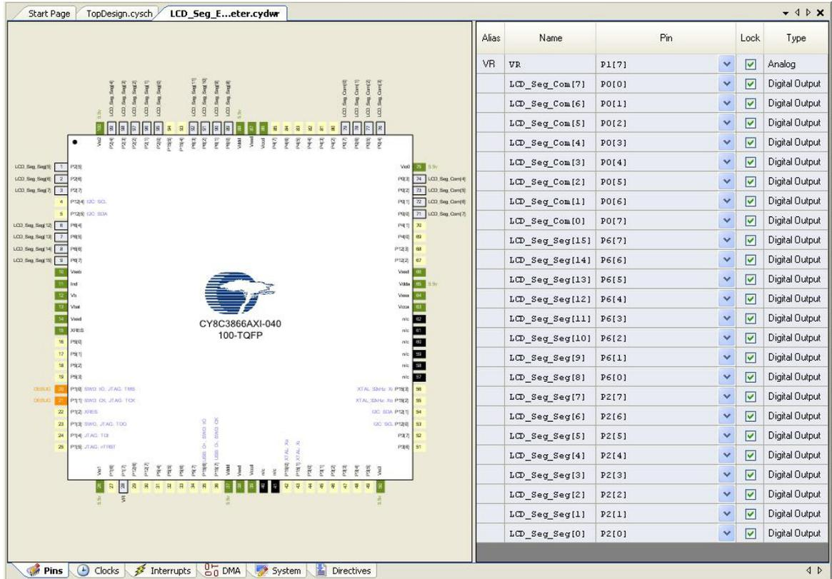
**Note** The pins for VR and SW1 must be reassigned to any other free GPIO when using Port A' and Port B. This is because P0\_2 pin used in both code examples for VR and SW1, is used for common lines.
