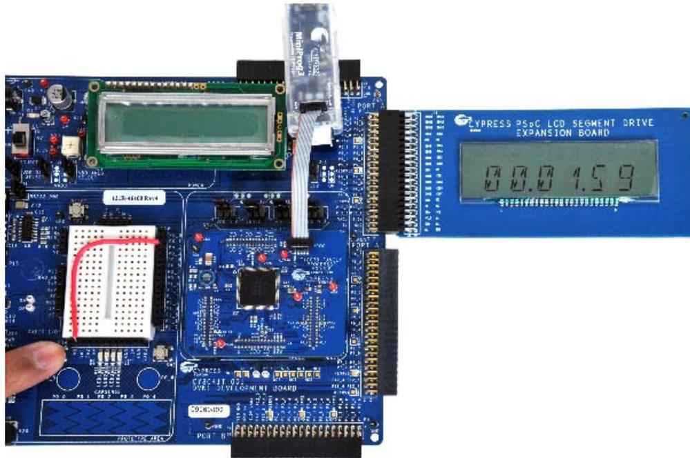
Pressing SW1 the first time starts the stopwatch and the values HH.MM.SS from the RTC are displayed on the LCD. The stopwatch increments every second. The second press stops the stopwatch and the value at which the watch stopped (HH.MM.SS) is displayed on the LCD. The third press of the switch resets the display to 00.00.00 (HH.MM.SS).
