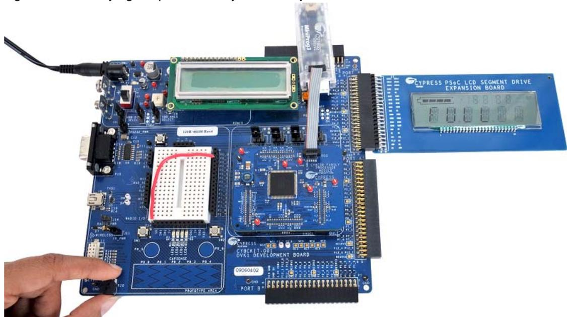
**Note** The best viewing angle is from 6 o'clock, according to the LCD glass characteristics.
