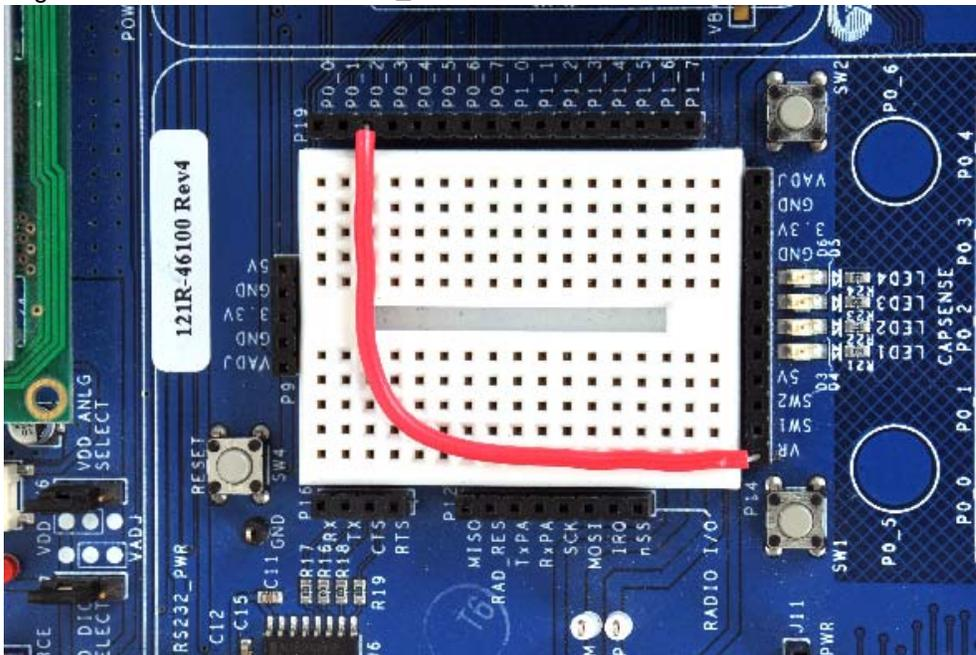
Power the VR by setting jumper J11 to the 'ON' position.
