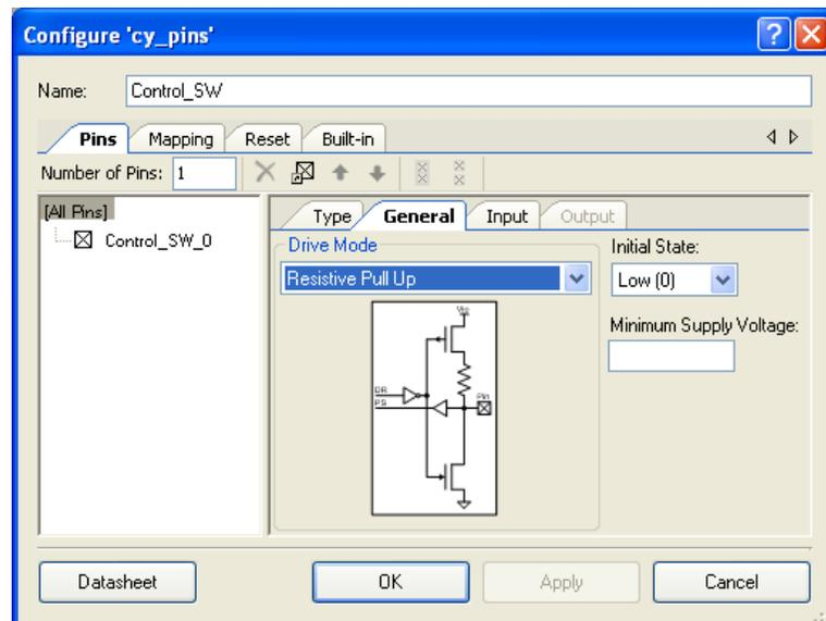
**Note** Pin assignment in both code examples is according to Port A of the DVK. Open the code example and change the pin assignment in PSoC Creator (.cydwr file) for Port A' or Port B according to [Table 4-2](#). The pin assignment for code example 1 is shown in [Figure 5-26](#).
