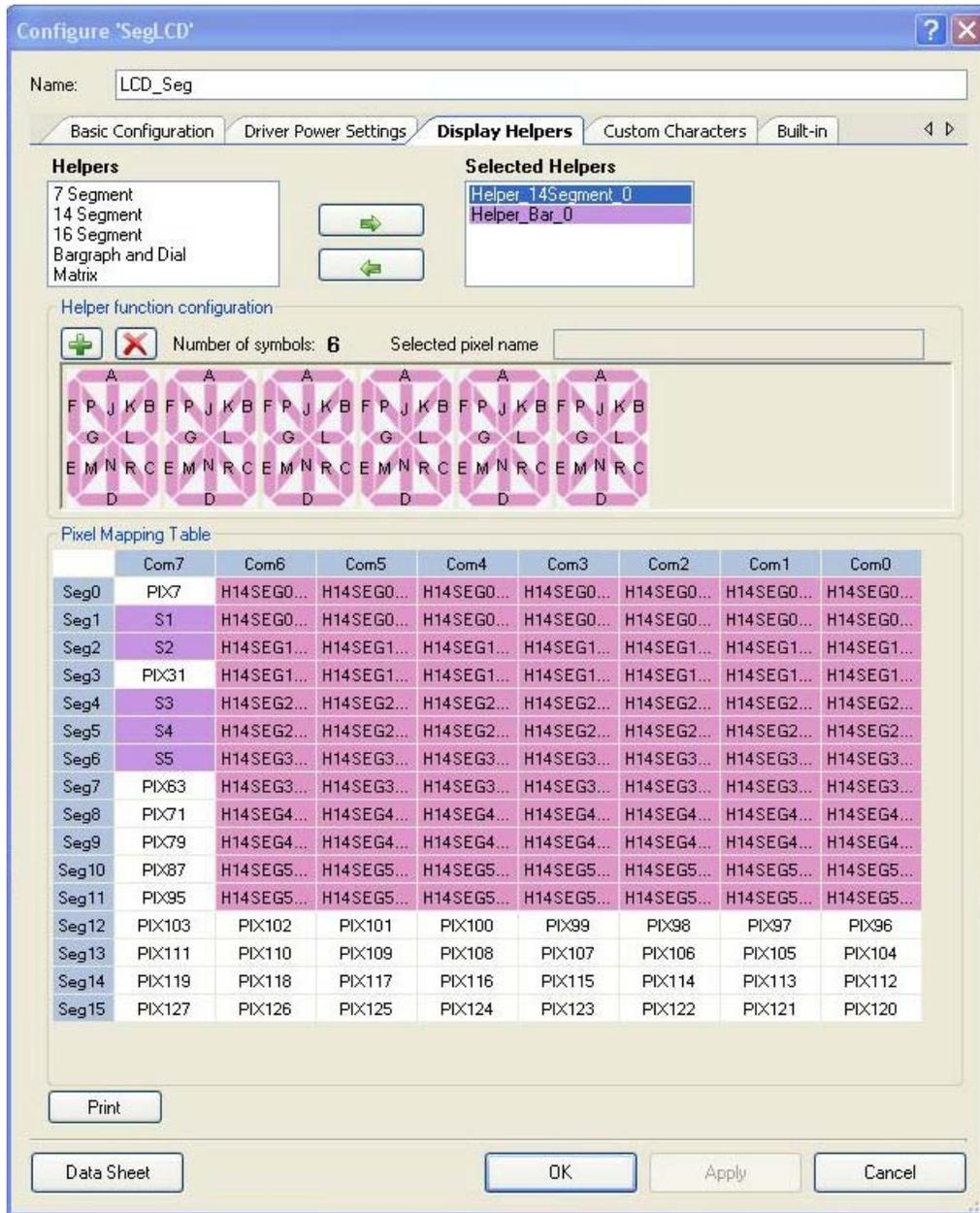
Figure 5-7. Bar Graph Helper for 5 Battery Indicator Segments
