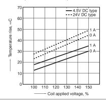
7. Ambient temperature characteristics Tested sample: AGN2004H, 6 pcs.
