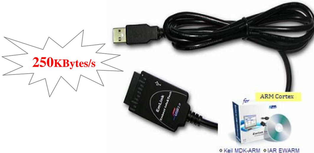
Emlink for ARM is a new-generation high-speed real time JTAG adapter, debugs the ARM Cortex-M3 processors through Keil Realview MDK and IAR EWARM. Emlink connects the JTAG interface from target board (ARM processors) to PC USB port, supports source level debugging and Flash programming.
