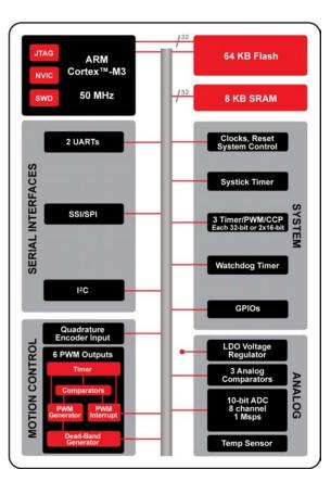
**LM3S800 Series Block Diagram.** This block diagram shows the superset of features for the LM3S800 series of microcontrollers.
