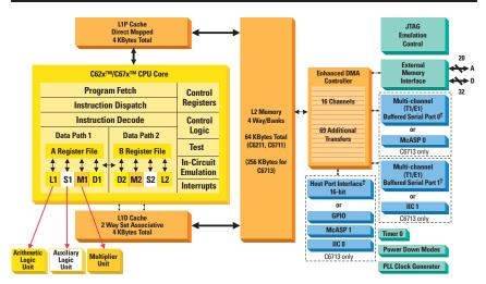
The C6713 DSP offers the audio customer base unparalleled levels of flexibility and performance. This superset of the C6711 and C6712 DSPs includes I<sup>2</sup>S, I<sup>2</sup>C and S/PDIF transmit support as well as enhanced memory space. Non-audio customers can also use this DSP as an upward migration path from the C6711 DSP.
