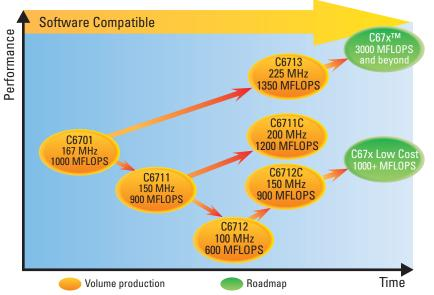
The TMS320C6713 DSP is the newest member of the C67x DSP generation. It features a performance of 1350 MFLOPS, 2 Mbits of on-chip SRAM and the new Multi-channel Audio Serial Port (McASP).
