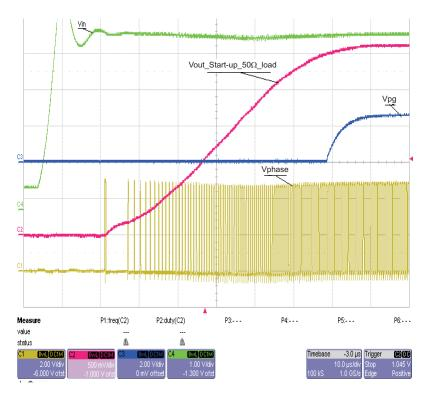
Figure 7. Start-up in PWM/PFM Mode. Vin = 5 V, Vout = 2.5 V, lout = 0.5 A; CH4 = Input Voltage; CH1 = Phase; CH2 = Output Voltage; CH3 = PG
