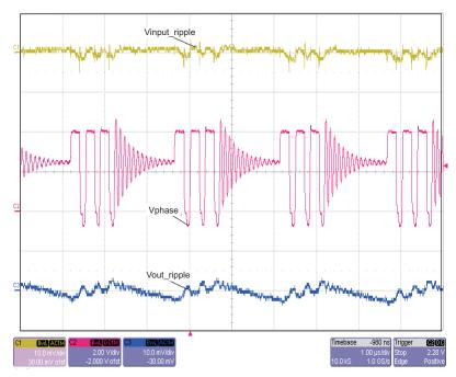
Figure 3. PFM Mode. Vin = 4 V, Vout = 2.5 V, lout = 25 mA. DCM Operation, Therefore PFM Mode CH1 = Input Ripple; CH2 = Phase; CH3 = Output Ripple
