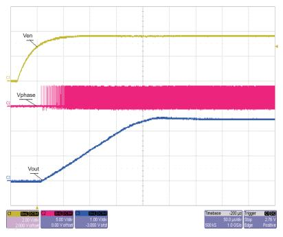
Figure 10. Power-up Output With EN pin. Vin = 4 V, Vout = 2.5 V, lout = 0.5 A; CH1 = Input Voltage; CH2 = Phase; CH3 = Output Voltage
