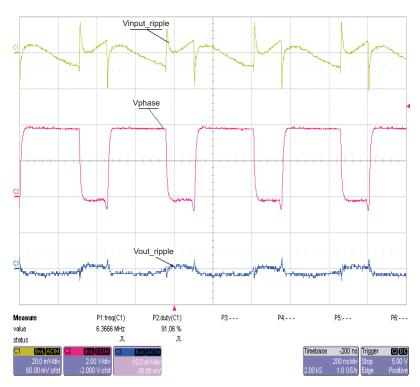
Figure 2. PWM Mode. Vin = 4 V, Vout = 2.5 V, lout = 0.5 A. CCM Operation, Therefore PWM Mode CH1 = Input Ripple; CH2 = Phase; CH3 = Output Ripple
