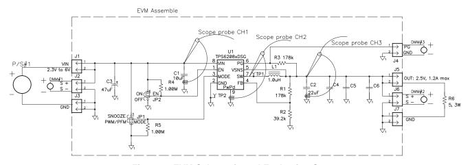
Figure 1. EVM Schematic and Evaluation Setup
