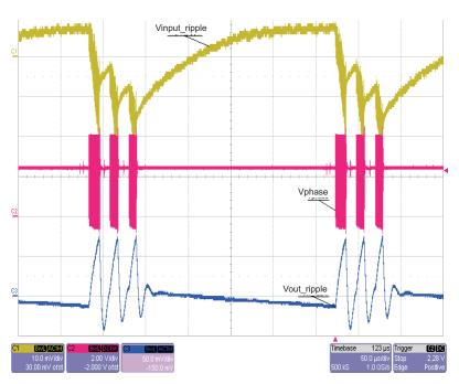
Figure 4. SNOOZE Mode. Vin = 4 V, Vout = 2.5 V, lout = 25 mA. CH1 = Input Ripple; CH2 = Phase; CH3 = Output Ripple
