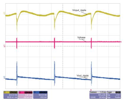
Figure 5. SNOOZE Mode. Vin = 4 V, Vout = 2.5 V, lout = 3 mA; CH1 = Input Ripple; CH2 = Phase; CH3 = Output Ripple
