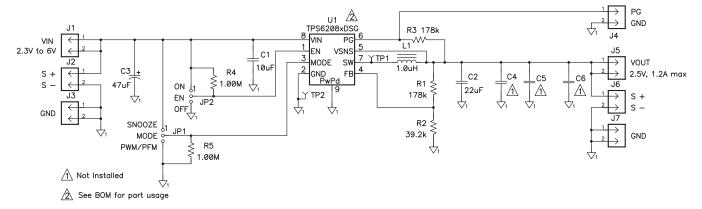
Figure 11. Schematic
