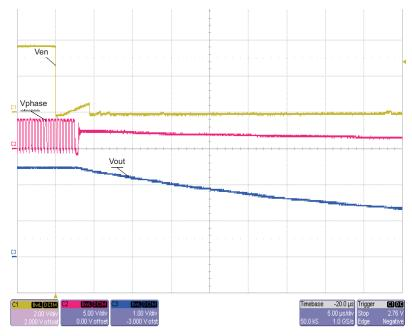
Figure 9. Shutdown Output With EN Pin. Vin = 4 V, Vout = 2.5 V, lout = 0.5 A; CH1 = Input Voltage; CH2 = Phase; CH3 = Output Voltage
