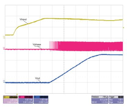
Figure 6. Start-up in PWM/PFM Mode. Vin = 4 V, Vout = 2.5 V, lout = 0.5 A; CH1 = Input Voltage; CH2 = Phase; CH3 = Output Voltage
