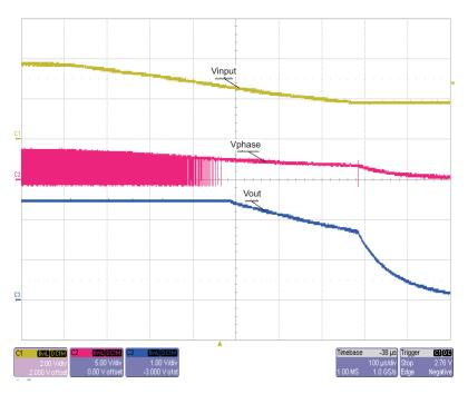
Figure 8. Power Down in PWM/PFM Mode, Vin = 4 V, Vout = 2.5 V, lout = 0.5 A; CH1 = Input Voltage; CH2 = Phase; CH3 = Output Voltage
