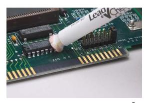
Rub the test area with an activated **LeadCheck® Swab**.
