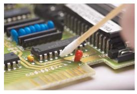
Vigorously rub a test area with the tip of a small swab. The diameter of the tip is about 3mm.
