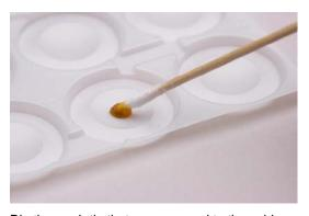
Dip the swab tip that was exposed to the solder into the drop of reactive dye.
