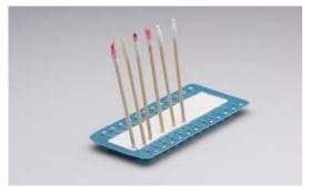
Dry swabs can be used on different areas of the board. Use the numbered clay tray to hold exposed swabs. Place a drop of dye from an activated LeadCheck<sup>®</sup> Swab either directly on the exposed swab or rub the exposed swab into a drop of dye on the tray. Positive swabs turn pink or red.
