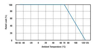
For resistors operated in ambient temperatures above 70°C, power rating must be derated in accordance with the curve.
