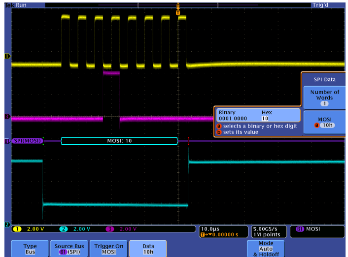
Triggering on a specific MOSI data value on the SPI bus.
