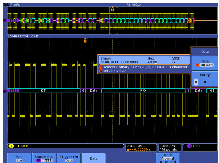
Triggering on a specific data value on the MIL-1553 bus.
