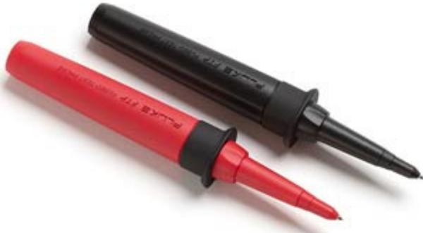
SureGrip Fused Test Probes with built-in replaceable fuses for additional measurement protection. If the probe fuse does blow, these fused test probes will still allow the meter to indicate live voltage, helping to prevent a possible misreading of no voltage present. These modular probes mount onto any standard modular test leads, for instance the Fluke TL221, TL222, or TL224. Rated to CAT III 1000V, these probes have removable tip guards for reduced probe tip exposure.
