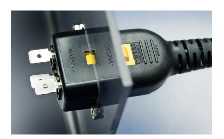
The lock is released by pressing a finger on the disengaging lever. This lever is easily identified due to its bright yellow color, a feature that also distinguishes this scheme from conventional pluggable power supply systems. The extraction force is at least 200 N.
