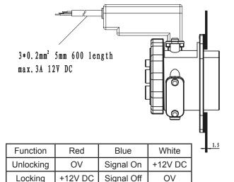
Actuate Solenoid Lock Using Single Pulse, Reverse / Changeover Polarity to Unlock
