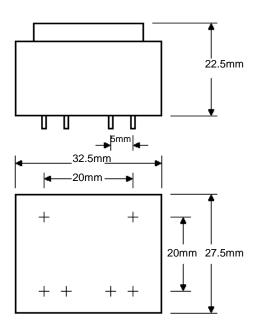
**DESCRIPTION**: 1.5VA Encapsulated Inherently Short Circuit Proof Transformer
