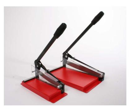
The DM9000 has a cutting capacity of 203mm (8") and is extremely compact with an overall height of only 575mm and a footprint of 335 X 140mm. It has a cutting bed of 110mm wide from the blade although wider material can be cut.
