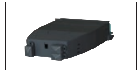
AX104617, FiberExpress Ultra HD Pre-Terminated Cassette, LC Duplex - MPO (m), 18 ports, 36 fibers, back view
