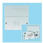
The NTE5A master socket provides a clear demarcation between the telephone operators network and the customer extension wiring via a removable connection unit (lower half). The product also provides line test, ringing components and over voltage protection. The NTE5A features a BT601A socket (4 wires connected) on the front for connection. tion of telephone apparatus as well as an IDC connection on the rear for extension wiring.
