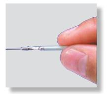
1. Grasp crimped contact approximately 1.0" (25.4mm) behind the contact barrel.
