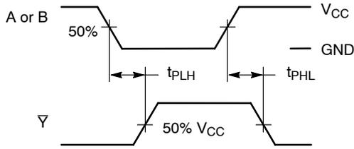
Figure 3. Switching Waveforms
