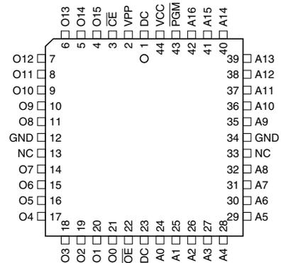
Note: Note: PLCC package pins 1 and 23 are Don't Connect.
