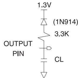
Note:  $CL = 100 \text{ pF}$  including jig capacitance, except for the -55 devices, where  $CL = 30 \text{ pF}$ .
