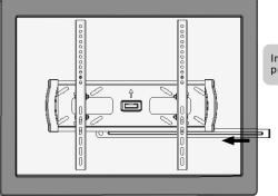
Insert the safety bar at the bottom of the mount to prevent the TV from being knocked off accidentally.
