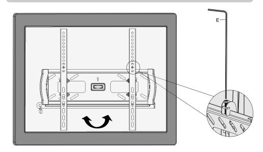
You can slightly adjust level for the display by tightening or loosening screws using a 5mm Allen key.
