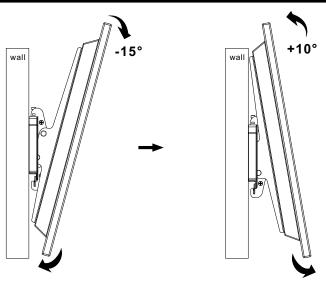
Push or pull from the top or bottom of the display to the desired angle.
