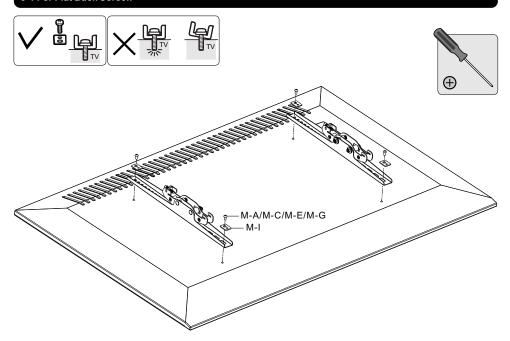
Tighten all screws but do not over tighten.
