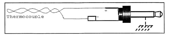
For K thermocouple – Connect Green cable to +
