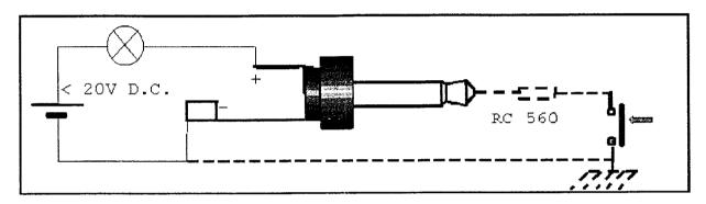
Alarm output: be sure not to overload this output - Maximum voltage: 20 Volts
