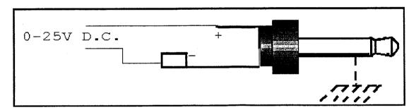
Voltage Input: Maximum voltage must not exceed 25 Volts
