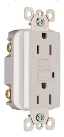
TradeMaster/Spec Grade GFCI Receptacle with high-impactresistant thermoplastic construction. It has SafeLock<sup>TM</sup> Protection: if critical components are damaged and ground fault protection is lost, power to receptacle is disconnected. It prevents the line-load reversal miswire: no power to the face or downstream receptacles if wired incorrectly. Its mounting screws are shipped captive in the device and wall plate for easier installation. 10kA SCCR, 15A 125VAC, White
