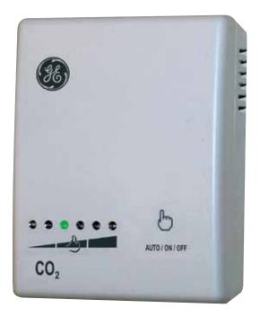
Unlike scientific displays, training to understand PPM values is not prerequisite with this innovative product. Indication shows under ventilation (red) or over ventilation (blue), which translates to low air quality (red) or too much energy being used to heat or cool unnecessary outside air (blue). In a heating only application the blue should be ignored if windows are opened to provide cooling.
