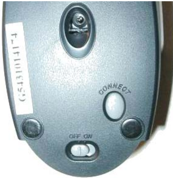
Figure 3-1. Bottom View Bind Button and On-Off Switch
