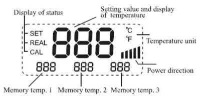
Display of status SET: Set Temperature REAL:Real Temperature CAL: Calibration Temperature
