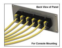
The Snap Strip is an alternate mounting method when two or more miniature panel jacks are to be installed in a row. Only a single rectangular opening is required to mount any even number of connectors. Just snap the MPJ connectors in and then snap the assembly into the panel. The black nylon Snap Strip accepts all calibrations of MPJ connectors.
