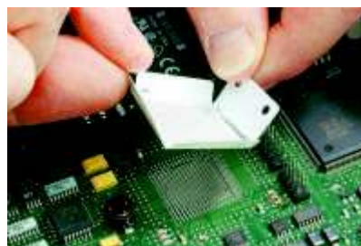
Step 5: Remove the stencil and save for another reuse or dispose.
