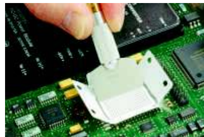
Step 4: Apply paste using a standard metal squeegee.
