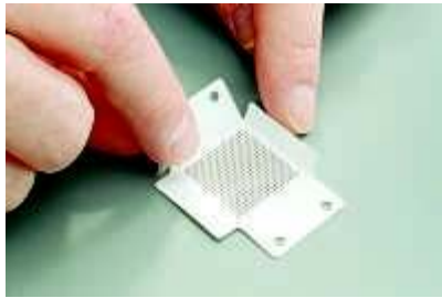
Step 1: Select the proper size and fold up the side tabs.
