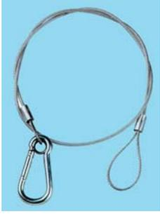
Used when rigging lighting effects these safety cables provide a secondary flexible coupling in addition to the regular fixing. Constructed from galvanised steel cable with spring-gate carbiner hooks. The cables are available in two weight capacities to better suit the application and each feature a PVC coating. Ideal for use on stage or in pubs/clubs.
