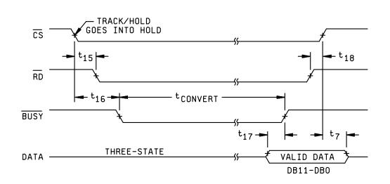
FIGURE 3. Mode 2 timing diagram, (12-bit parallel read).
