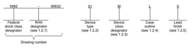
1.2.1 <u>RHA designator</u>. Device classes Q and V RHA marked devices meet the MIL-PRF-38535 specified RHA levels and are marked with the appropriate RHA designator. Device class M RHA marked devices meet the MIL-PRF-38535, appendix A specified RHA levels and are marked with the appropriate RHA designator. A dash (-) indicates a non-RHA device.
