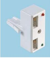
This unit is designed to prevent eaves dropping or dialling across calls when an extension line is fitted. A switching device is incorporated in the adaptor together with LED indicators. When one of the telephones is in use, the unit blocks interference and eaves dropping from the other telephone. This is indicated through the LED.
