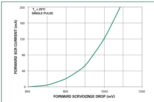
**Figure 3: High Current SCR Forward Voltage Drop Curve**
