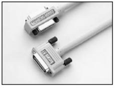
Model 7006-\*: Single-shielded GPIB cable terminated with one feed through style and one straight on IEEE-488 connector. The mating thumb screws are metric. 7006-1 1m (3.3 ft) 7006-2 2m (6.6 ft)
